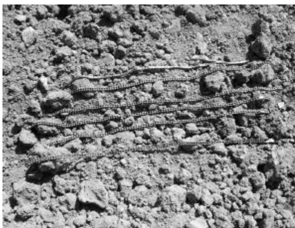
Figure 2.1 Chain set used to measure soil surface roughness (Moreno et al., 2010)
