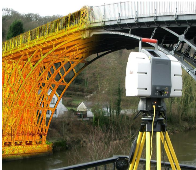
Figure 2.5 Commercial terrestrial laser scanner that provides accurate 3-D model of a bridge structure (RUDI, 2014)
