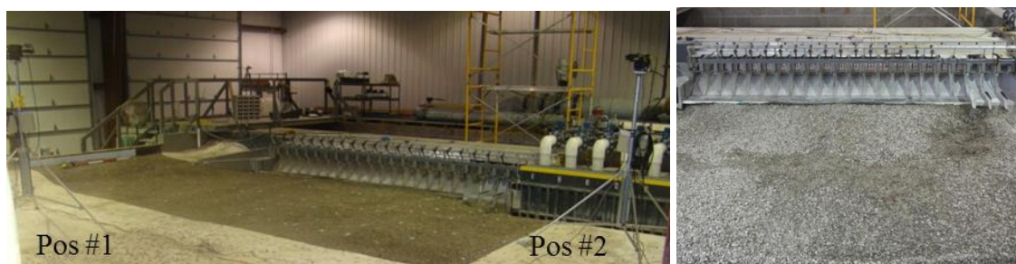
Figure A.1 Photographs of initial bathymetry modeled from a multi-beam hydrographic survey (left) and final bathymetry after the PMF (right)
