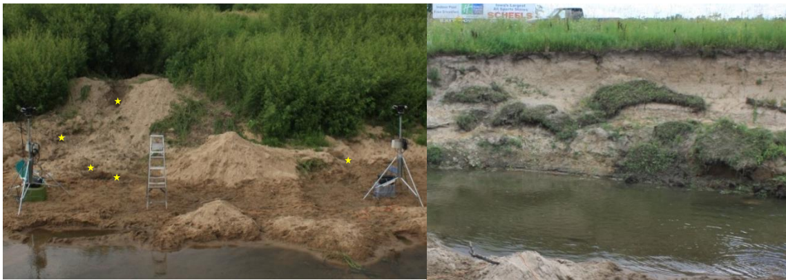
Figure B.3 Image of field equipment with 5 of 7 GCPs marked with a yellow star (left) and image of profiled streambank with trimmed vegetation (right)
