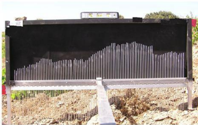
Figure 2.2 Pin meter used to measure soil topography (Moran)
