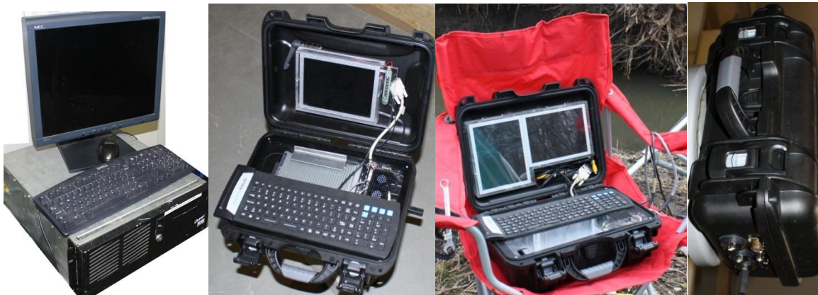
Figure 3.3 Bulky monitor/CPU (left), weatherized computer (left-center), weatherized computer with monitor for camera (right-center), and side view of closed box (right)
